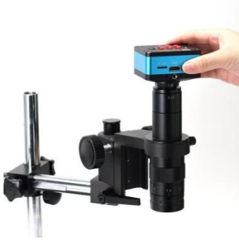
Mount the HDMI Industrial camera
